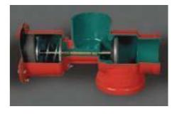
The Yardney patented cast-iron backwash valve is the only valve in the industry designed as standard equipment to be 100% field serviceable with basic hand tools and includes a grease fitting for valve shaft lubrication. Valves feature fusion epoxy lining and the valve shaft and seal retainers are noncorrosive stainless steel with durable, molded polyurethane seals.
