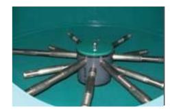
The underdrain system features a lateral design of high strength stainless steel wedgewire, producing a pressure drop of only 4 psi, and will withstand collapse pressure in excess of 600 psi.
